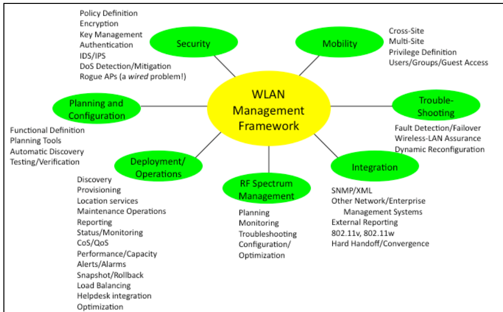
Figure 2 – A partial list of the functions of the management plane in a WLAN architecture. Management must be centralized, and the importance of these capabilities in successful installations cannot be overestimated. Source: Farpoint Group.
